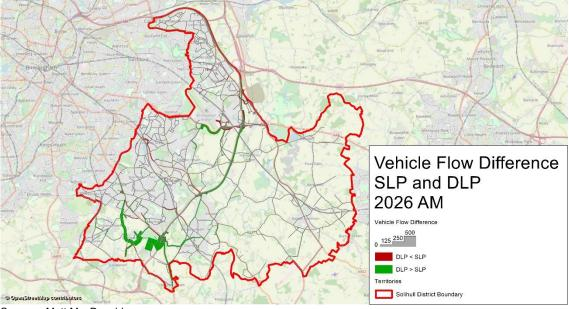
Figure B.1: Vehicle Flow Differences: SLP and DLP 2026 AM
