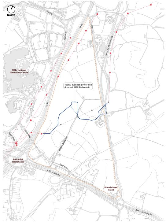
Current pylons and overhead power lines (proposed undergrounding of E-W route shown in grey)
