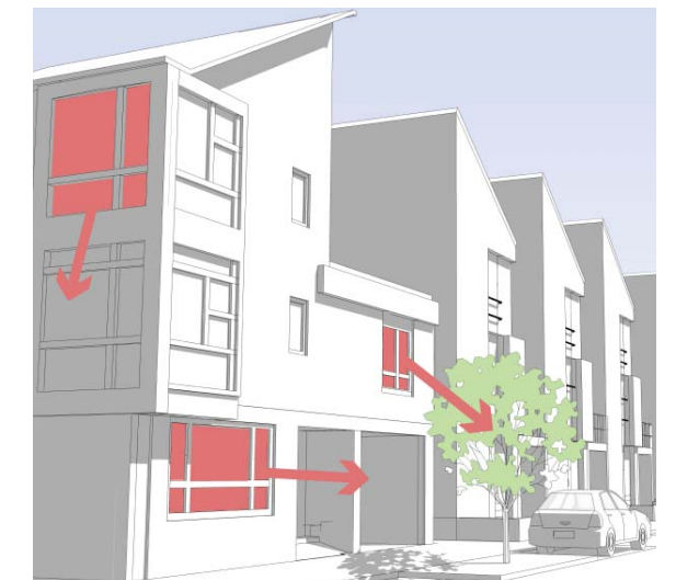
Active Frontage enables good natural surveillance of the street
