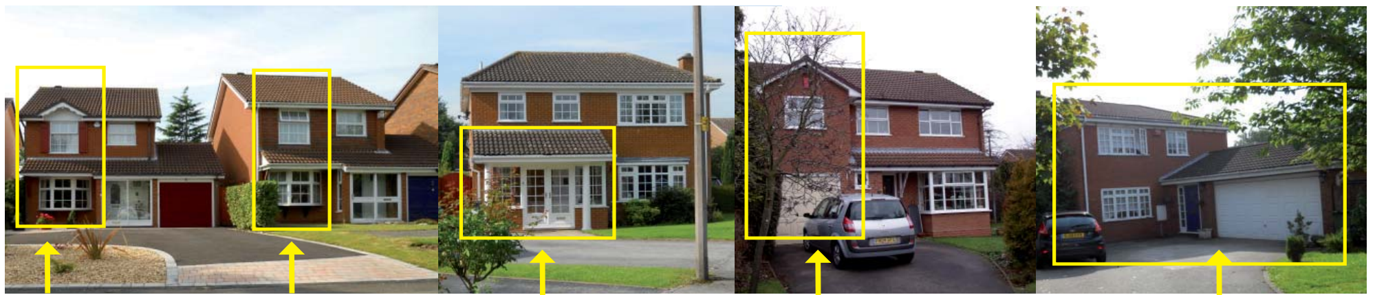
Small detached properties have pitched roofs which house the porch and garage. Small gable features above first floor windows add variety to the streetscene. Roof lines are hipped and do not have chimneys.
