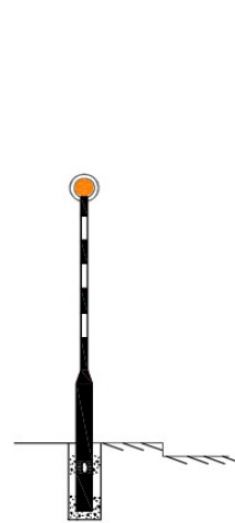
TYPE 3 BEACON : Beacon column mounted
