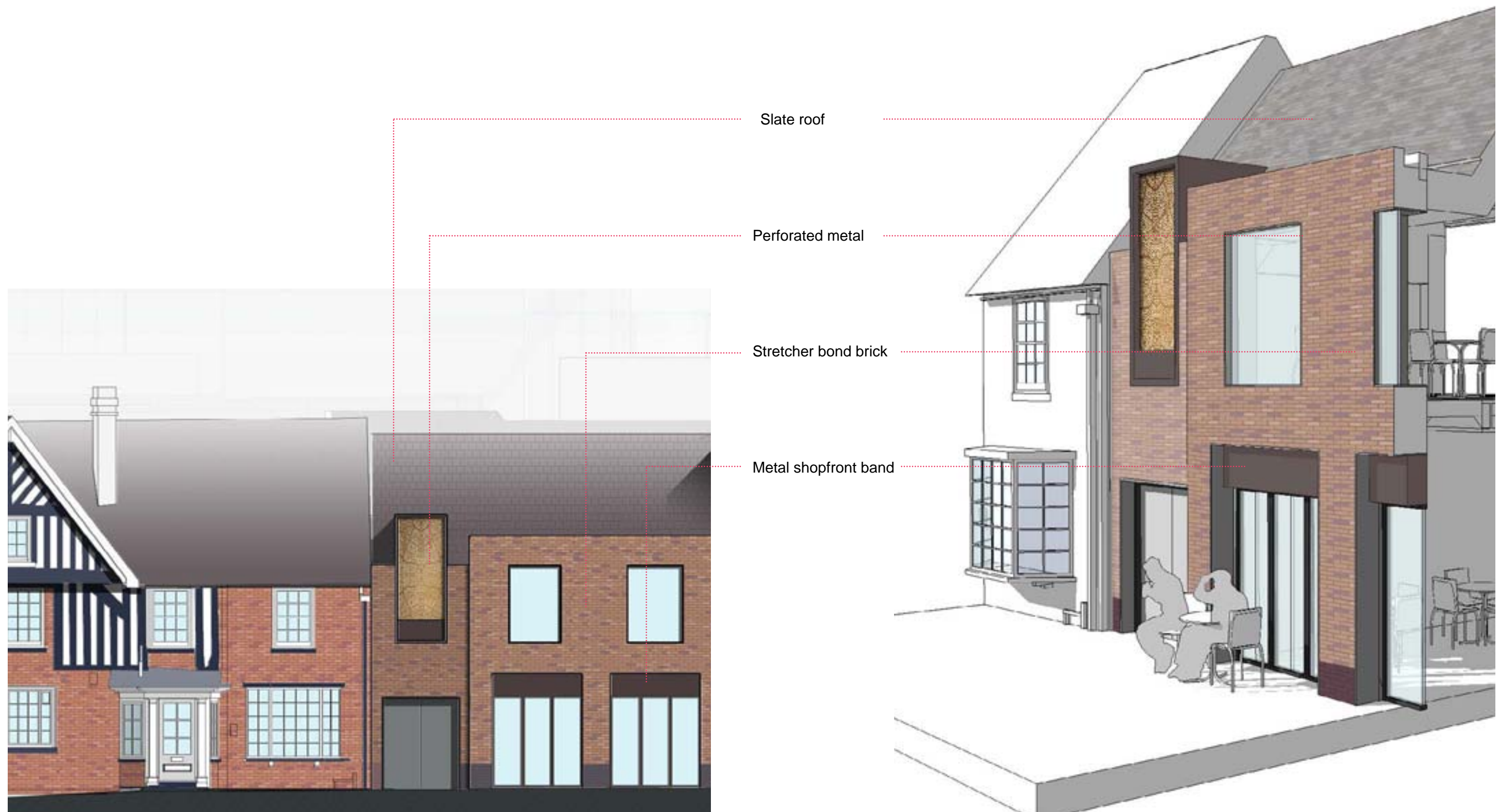
Figure 3.4.3.22 Elevation of 158 High Street connection
