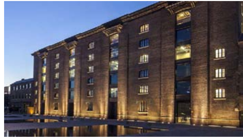
Figure 4.9.7.3 Lighting grazing up a wall installation example
